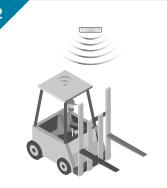
Use Impinj readers and gateways installed in doorways, ceilings, or rooms to wirelessly identify and locate items in all company facilities.
